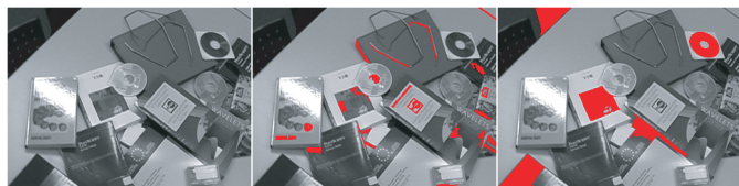
Fig. 6. Typical output images from demonstrator. To the left is the original image. The result of different max- and min-size settings are shown in the other images, red indicates MSERs. Detected MSER sizes are (middle) 64-200 and (right) 800-1500 pixels. (The MSERs are only visible in color.)
